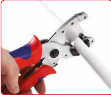
1. Cut the pipe at a 90° angle.
