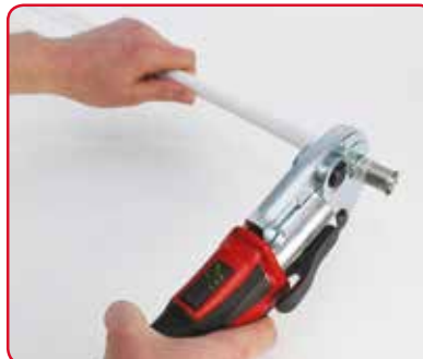
5. Using a Maincor Pressing Tool or Mini Pressing Tool, make the connection.
